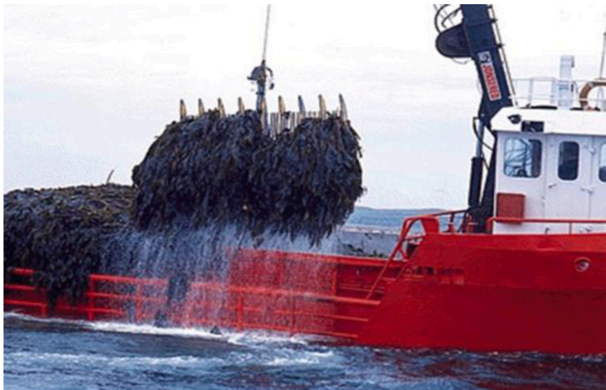
Figure 2. Norwegian kelp harvester in operation, source Vea & Ask, 2011.
