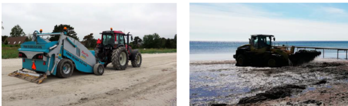
Figure 3. Beach cleaning machine (left panel) and loader tractor collecting beach cast in water (right panel) in Denmark, source Lybæk & Kjær, 2023.
